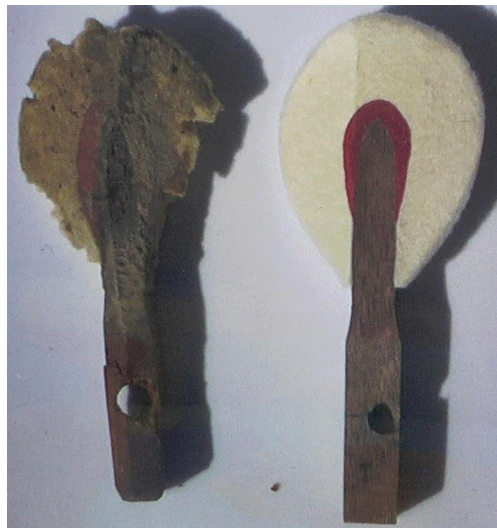
Square Piano Hammers sample new hammer
